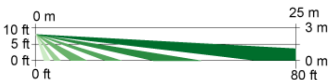
Side View Optional Barrier Coverage: 15 m to 25 m x 5 m (50 ft to 80 ft x 16 ft)
